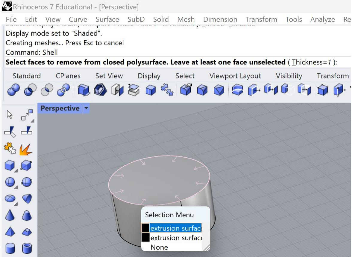
7. **Select at least one face.** Then, you can **type in a number** to change the thickness of the remaining walls. I typed in 2.
