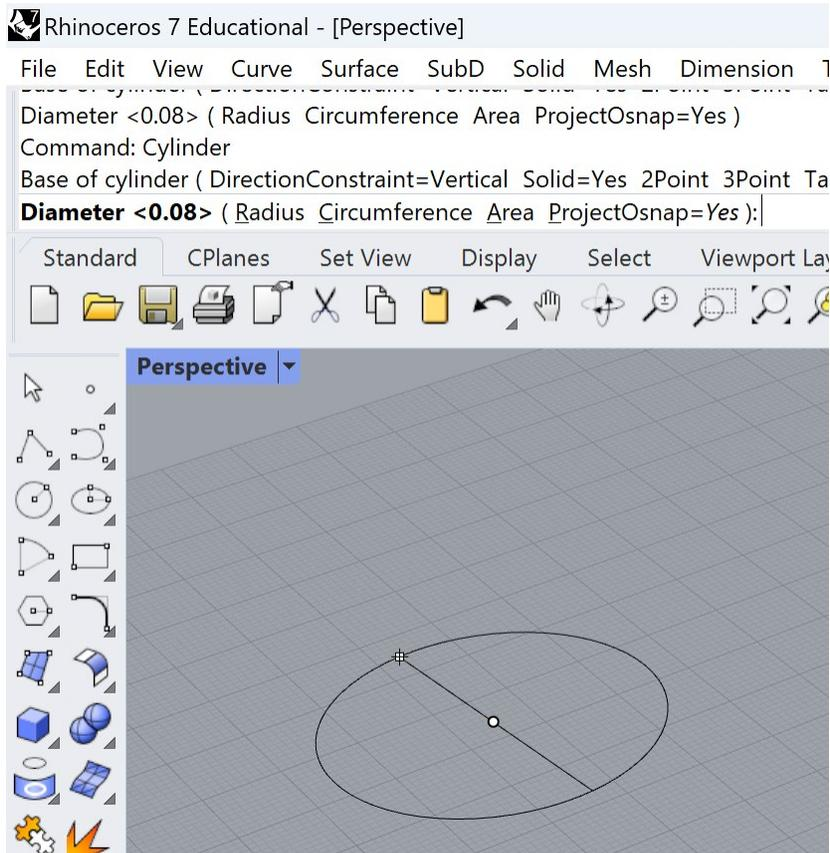
4. Read the command bar again and select a height for the cylinder. Once again, you can either **pick a height** or **type in a specific height**.
