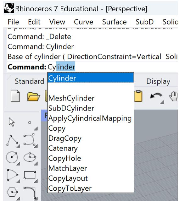
2. Read the command bar to figure out what to do next. In this case, **pick a point** to be the base of the cylinder.
