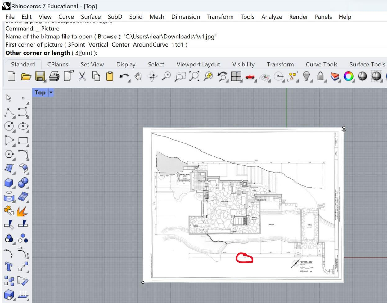
Look at your image to find any sort of scale indicator. It is usually helpful to pick a longer dimension if possible. For mine, I am going to use the dimension at the bottom that says 98'3," which is circled in red above.
