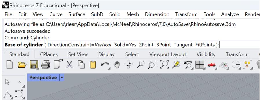
3. Read the command bar again and select a diameter for the base of the cylinder. You can either **select a point on the grid** or **type a number** to create a specific diameter. Notice that there are other options in the command bar, for example **“Radius.”** If you click on radius, you can do this step by selecting a radius for the cylinder instead of a diameter.
